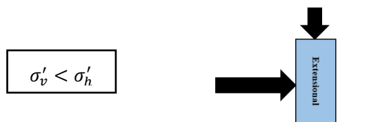
Fig.5.2 (a) Extensional loading condition (reducing \sigma'_v under constant \sigma'_h )
