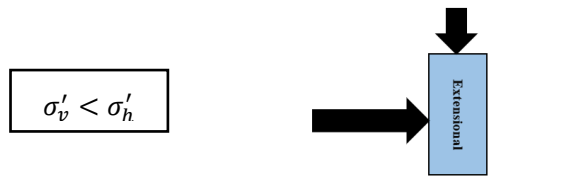
Fig.4.1 (a) Extensional loading condition (reducing \sigma'_v under constant \sigma'_h )
